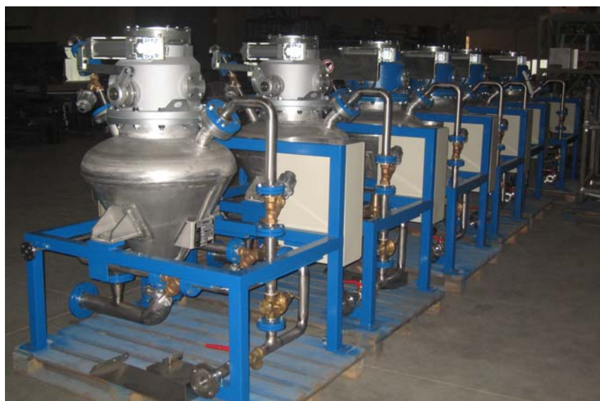
▶ MAB – PULSVEYOR Unit type PVE 50 for conveying POLYETHYLENE chips at 8 t/hr.
