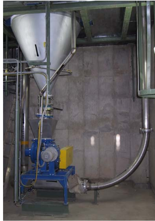
Rotary valve VRP-HP for PTA conveying system: 15 t/hr - 160 m
